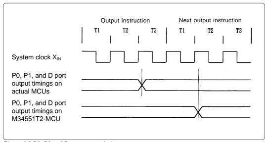
Figure 6.1 P0, P1 and D port output timings
